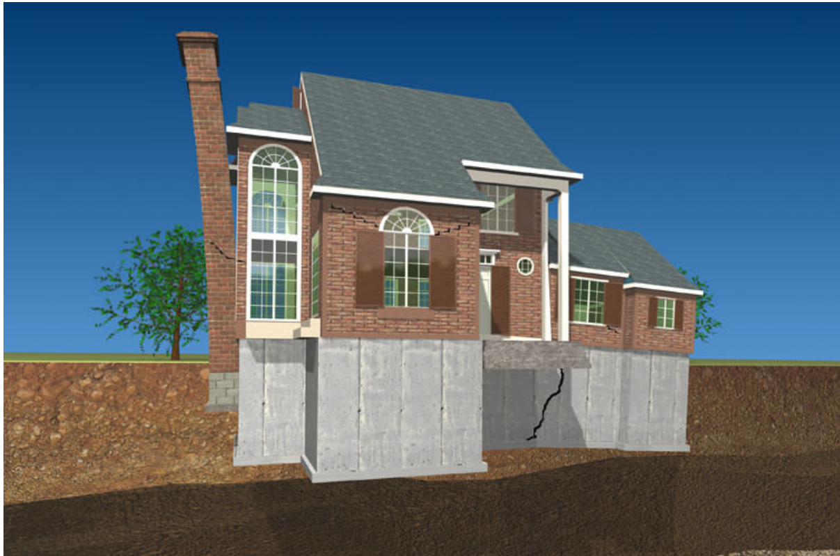
Figure 15: Image showing example of foundation sinking (credit: www.clarkebasementsystems.com )
