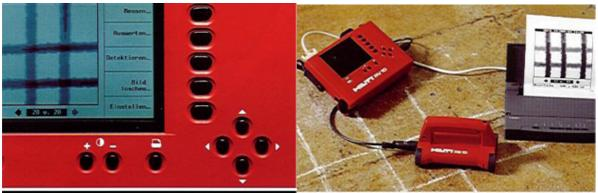
Figure 46: Ferro- scan used for deducting iron bar location (credit: TESRA ppt)
