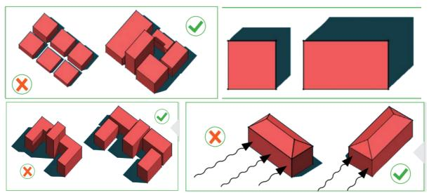
Figure 62: Disaster resilient building design pattern (credit: TESRA ppt)
