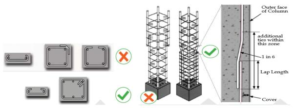
Figure 67: Reinforcement pattern in column and bar bending details (credit: TESRA ppt)
