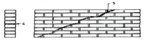
1B Cement mortar and flat chips in wide cracks
