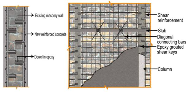
Figure 24: detail of retrofitting procedure for Stone wall (credit: TESRA ppt)
