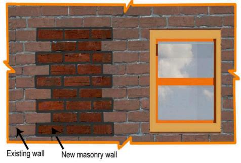
Figure 40: Closing of existing opening (credit:TESRA ppt)
