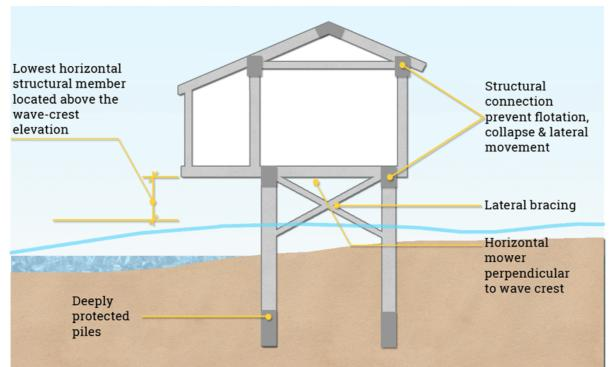
Figure 57: Image showing introduction of bracings between columns (credit: andhitapradipta.github.io)
