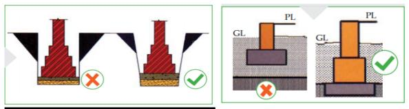
Figure 63: Foundation design and execution
