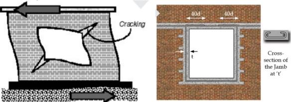
Figure 66: Protect Openings with Reinforced Band all around as shown.
