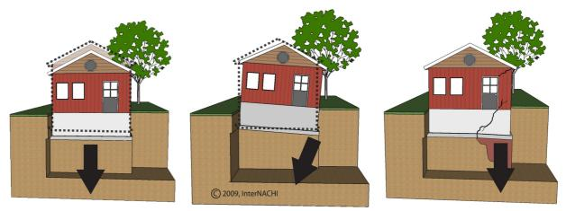
Figure 56: Image showing ground settlement pattern due to flood (credit:www.nachi.org)
