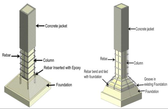
Figure 28: Jacketing of column and foundation (credit: TESRA ppt)
