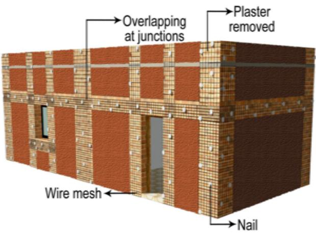
Figure 41: Installation of wire mesh around opening (credit: TESRA ppt)
