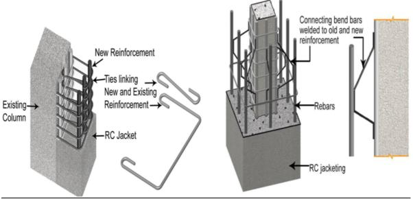
Figure 29: RCC jacketing of existing column (credit: TESRA ppt)
