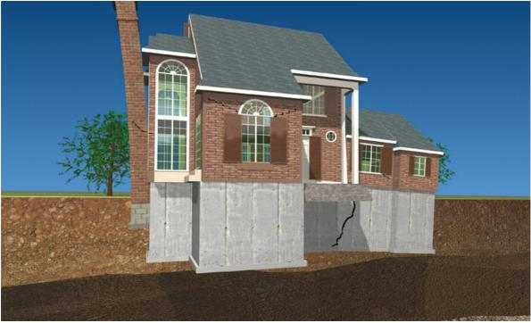
Figure 17: Image showing example of foundation sinking (credit: www.clarkebasementsystems.com)
