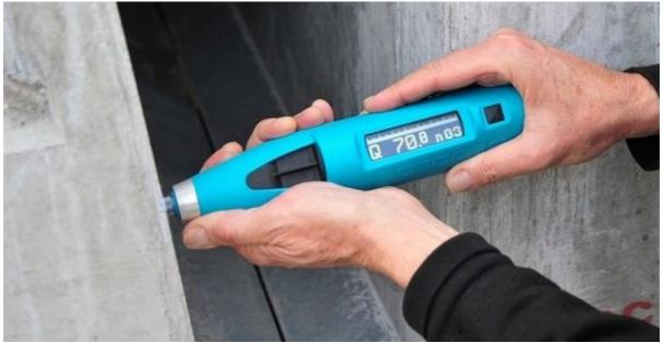
Figure 51: Re-bound hammer testing of concrete element (credit: gharpedia.com)
