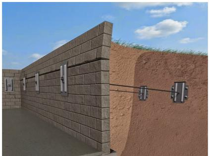
Figure 61: retrofitting using steel plates for basements (credit: TESRA ppt)
