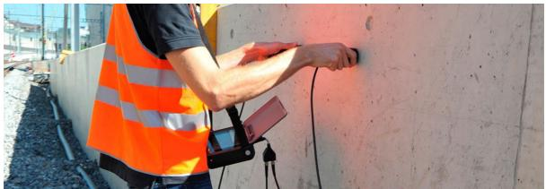
Figure 50: UPV testing of concrete element (credit: gharpedia.com)
