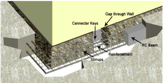
Figure 19: Strengthening of Foundation using RCC frame
