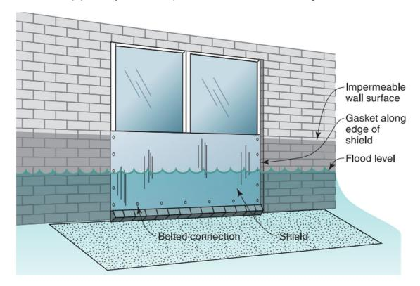
Figure 58: Image showing introduction of Temporary support to avoid flood water (credit: andhitapradipta.github.io)
