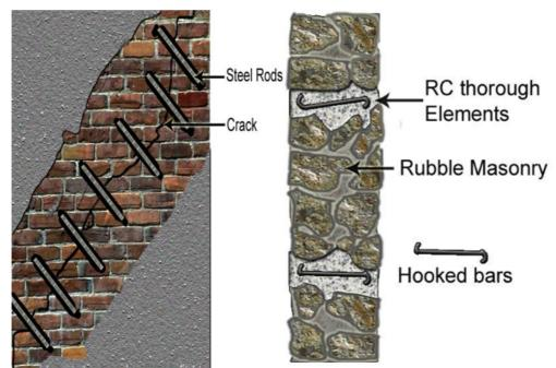
Figure 22: crack repair using 6 mm iron bars (left) and Hook bars in stone masonry wall (right)
