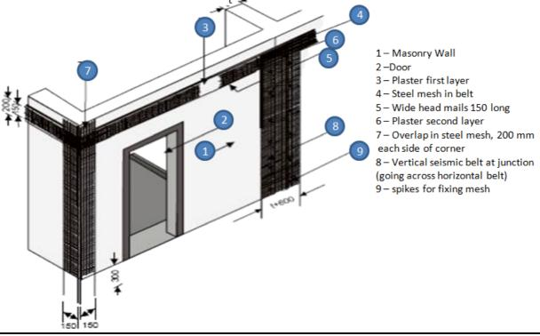
Figure 16: Image showing example of Retrofitting of using wire mesh installation (credit: urbansolutionsbd.blogspot.com)
