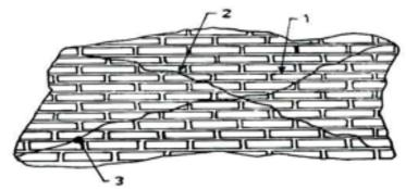
1A Grout or epoxy injection in cracks
