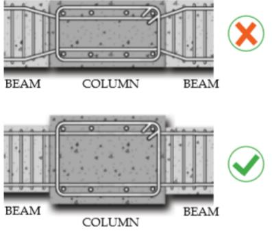
Figure 68: Reinforcement pattern on beam column joints (credit: TESRA ppt)
