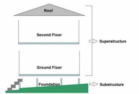
Figure 7: schematic diagram of building structure (credit: theconstructor.org)
