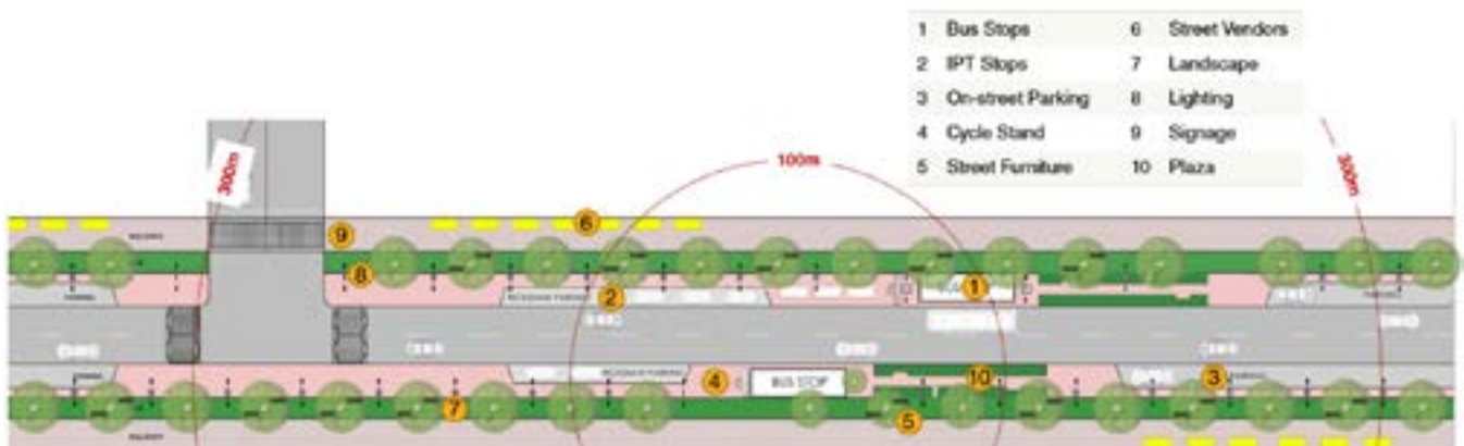
FIGURE 3.2 Complete Street design elements
