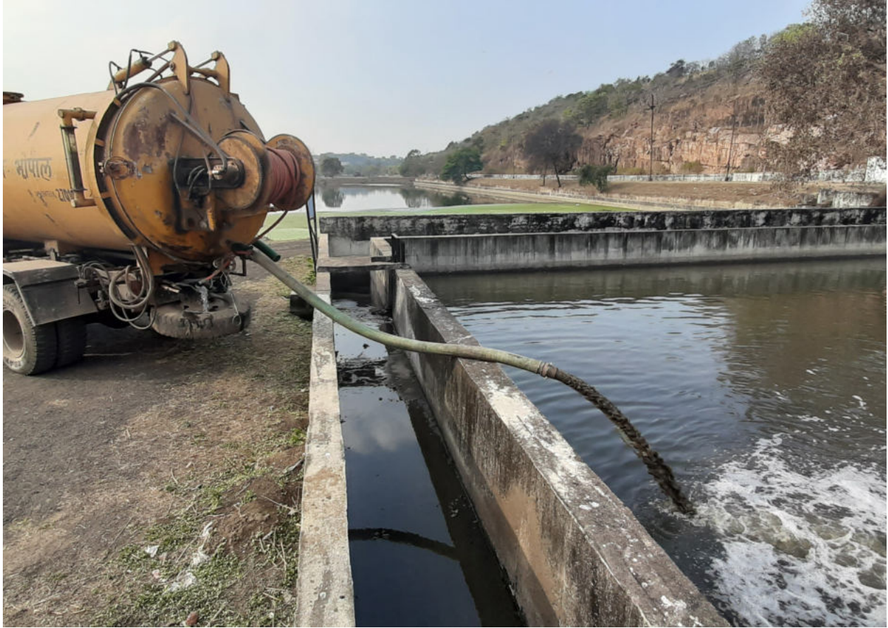
Image 4.10: Vacuum tanker emptying faecal sludge collected from onsite sanitation facilities at Kotra STP
